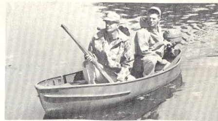
Retriever —Open model with same hull as Ducker. Has fantail mount for motors up to 3 horsepower. Recommended for use on small sheltered water. Very easy to row. See specifications.
