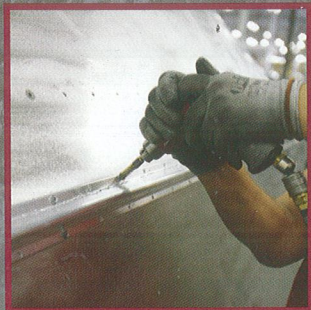
Top-quality aluminum hulls with larger aircraft-grade rivets for longevity
