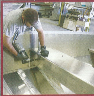
Durable wood-free, heavy-gauge aluminum seating and stringers
