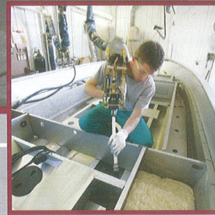
Gas-resistant expansion foam increases buoyancy and quiets the ride
