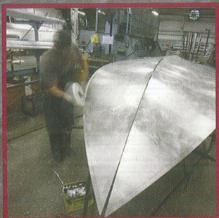
One-piece, single-sheet aluminum finely cut and shaped for the greatest possible inherent strength
